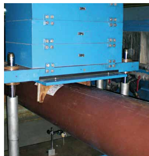
Tests for the determination of the pressure jetting resistance (picture top and centre) and longitudinal bending (picture bottom)
